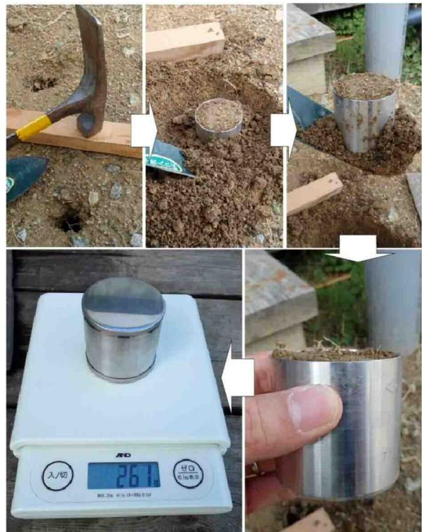
Fig.4 Unit weight test using circular cylinder
